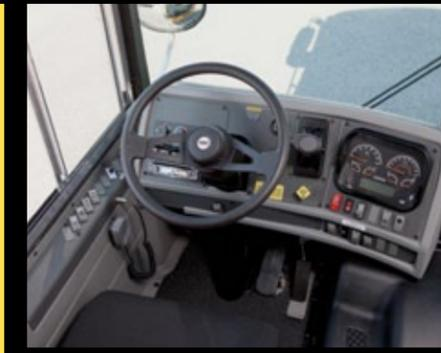
We've designed the cockpit to provide superior ergonomics and ease of operation. Switches are grouped and placed forward of the centerline of the driver's window. Heater and radio controls also are within reach.
