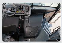
Engine access provides wider aisle for passenger loading and tool free access for serviceability.
