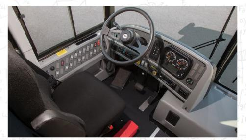
Every bus driver is different. The offset gauge cluster and the optional adjustable pedals make driving easier and safer for drivers of every shape and size. The standard tilt/telescoping steering wheel makes driving more comfortable for drivers.
