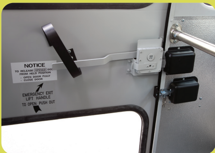
Vandalock - rear door vandal and interlock system
