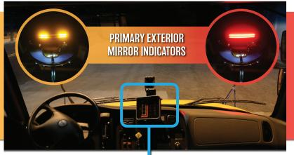
The Stage 2 indicator glows RED indicating there is a pedestrian in the CRITICAL ZONE which is less than 6 ft from the bus.
