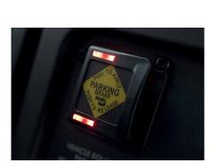
Intellipark parking brake technology helps prevent rollaway crashes due to drivers exiting their vehicles without setting the brake
