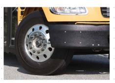
A wheel cut up to 55\* degrees for enhanced maneuverability. Bumpers are also available with corrosion protection.
