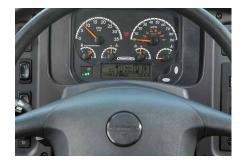
A non-reflective instrument panel features easy-to-read, LED-backlit gauges
