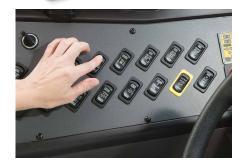
A multiplex-wired Smart Switch system offers easy access to switches and is designed to meet drivers' preferences without re-wiring
