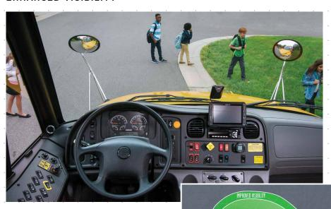
The C2 looks different because it is different. It was designed for maximum visibility and safety. The panoramic view, low sloping hood, low instrument panel and A-pillar windows result in the largest visibility footprint in the Type C category. The C2 also features large passenger windows that are easy to remove in case of an emergency.
