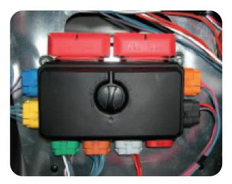
Multiplex wiring system allows multiple electronic messages to travel through the same datalink wire
